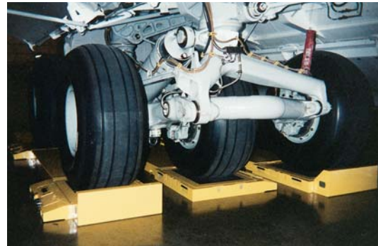
Hydraulic Jacking and High Capacity options used for Boeing and USAF C-17 Globemaster weighings.
