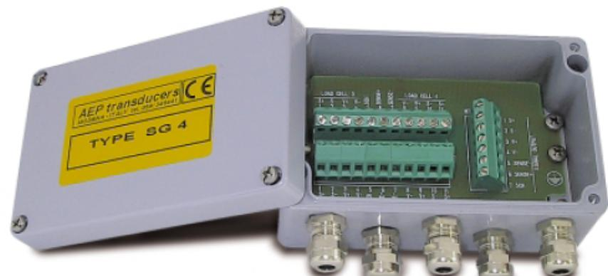
*SG4 junction box is used to make weighing, dosing and plants controlling easier, whenever connecting load cells in parallel is necessary, in order to have a single output signal which represents the sum of the signals of connected load cells. To realise connection of load cells in parallel, five PHOENIX terminal boards with screw-type clamping have been arranged and they are used to perform electrical connections of both input and output cables.*
