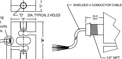
Cable restraint and sealing configuration for ZX-250, ZX-500, and ZX-1000 load cells and metric thread models.
