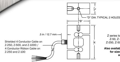
Z series load cell cable lengths: Z-50, Z-100 = 2.5 ft / 76 cm Z-250, Z-500, Z1000 = 30 ft / 9 m
