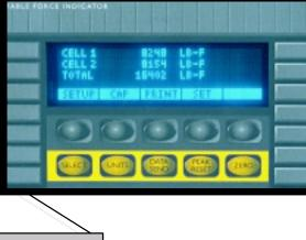
Wizard can be programmed to let operators read total weight of two load cells. It can use the load cell output for system control; it can shut down an overloaded system. Or you may wish to monitor the two load cells and automatically register the difference between the two for an early warning of uneven loading.
