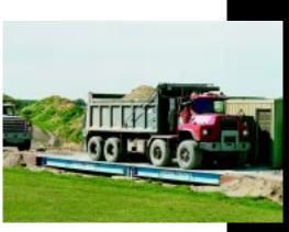
The WI-152 Indicator goes to work equally well with a truck scale at a remote site or a portable bench scale in a warehouse. Its 6-volt version. with D-cell battery pack includes a "sleep mode" which extends battery life to 2,300 hours depending on the system.
