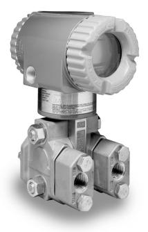
Viatran's Model IDP10 uses silicon sensor technology and microprocessor based electronics to provide a transmitter with exceptional accuracy and reliability. The modular electronics are housed in a durable NEMA 4X housing with corrosion-resistant epoxy coating. A stainless steel housing is available optionally for extremely corrosive and offshore applications. The electronics housing is fully rotatable and has two conduit entrances, allowing fully flexible installation.
