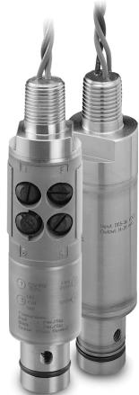
Viatran's Models 553 and 554 are designed for new and retrofit applications in the pulp and paper industry. The flush-mount units are available in a one-inch O-Ring design, compatible with 1" PMC process connection. The bonded foil sensor has no oil fill which means easy cleaning and no damage to the unit or its performance.
