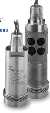
Viatran's Model 550 and 551 are the most rugged transmitters available for the pulp and paper industry. With a standard M44 X 1.25 flush pressure fitting (1-1/2" NPT optional) and 17-4PH NACE diaphragm they are ideal for use with the corrosive media that accumulates and clogs standard fittings. Unlike capacitance or micro-machined silicon sensors, Viatran's flush bonded foil sensor has no oil fill which means easy cleaning with no damage to the unit or its performance.
