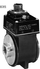
Viatran's "76" Series is a small size, low range differential pressure transmitter that is extremely accurate. Measuring 3.75" in height and 2.25" in width, this unit is one of the smallest wet/wet differential pressure transmitters available.
