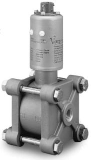
Viatran's "74" Series differential pressure transmitters are extremely accurate and durable units, designed specifically for test applications. The variable capacitance sensing technology provides extremely high overpressure protection, and long range stability, as well as high accuracy of 0.15% BFSL.
